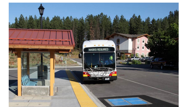
EV bus charger example. Photo: Momentum Dynamics Corp.
