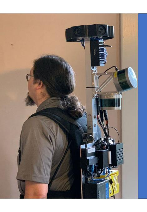
Scan the Station using LiDAR scanning technology
