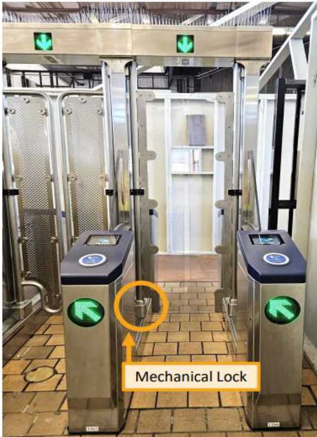
Mechanical Locks Implemented across all 715 Gates
