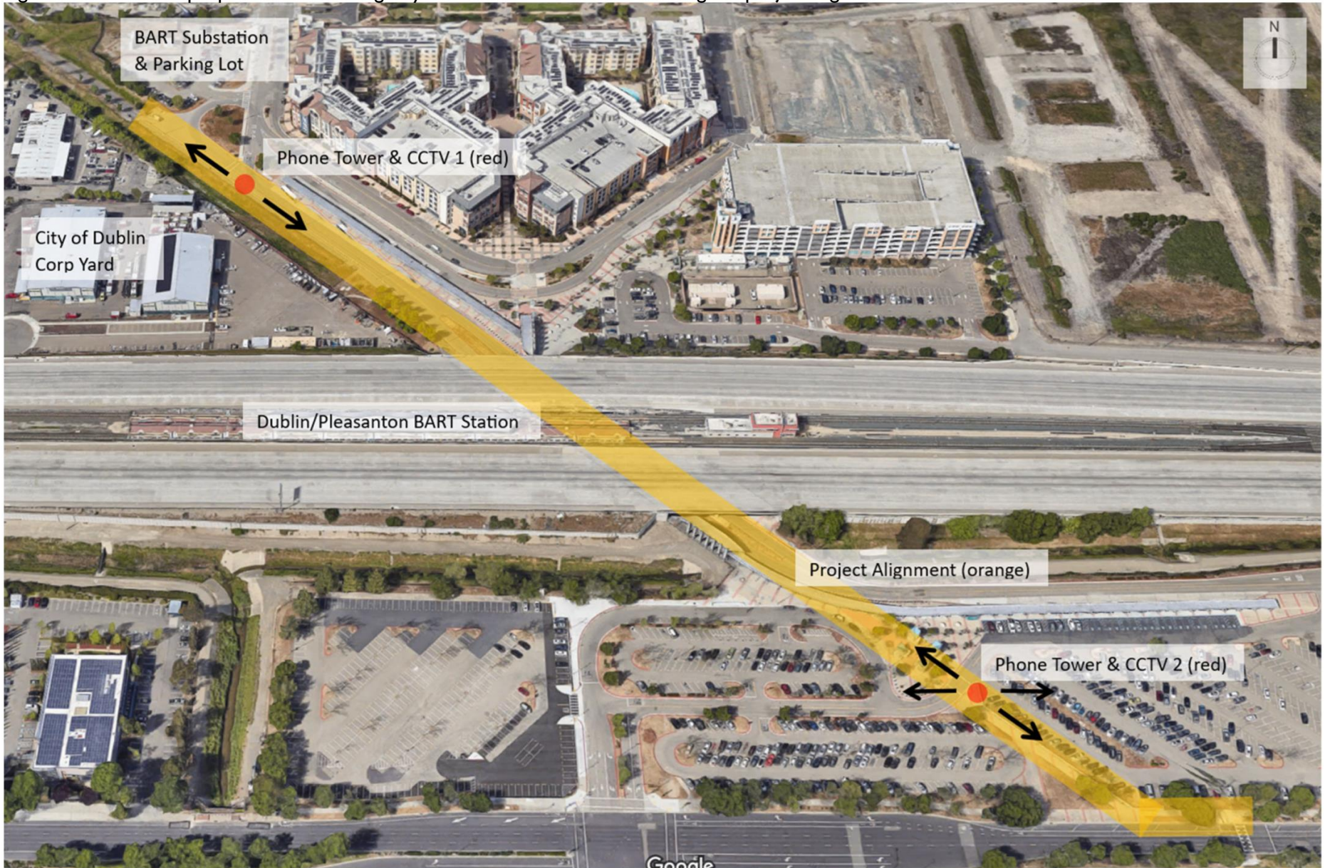
Figure I: Locations of proposed Public Emergency Phone Towers with CCTV along the project alignment
